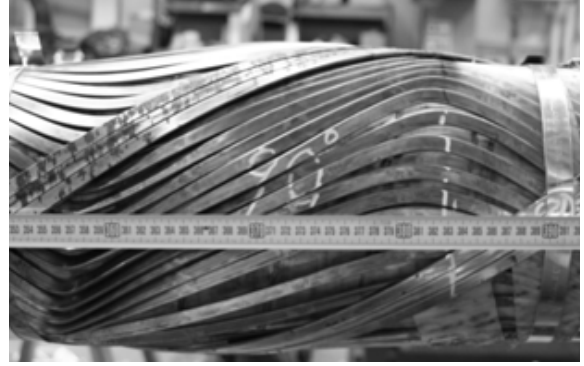
FIGURE 3. Lateral buckling in the inner layer of tensile armour wires, generated by NKT-Flexibles by laboratory testing
