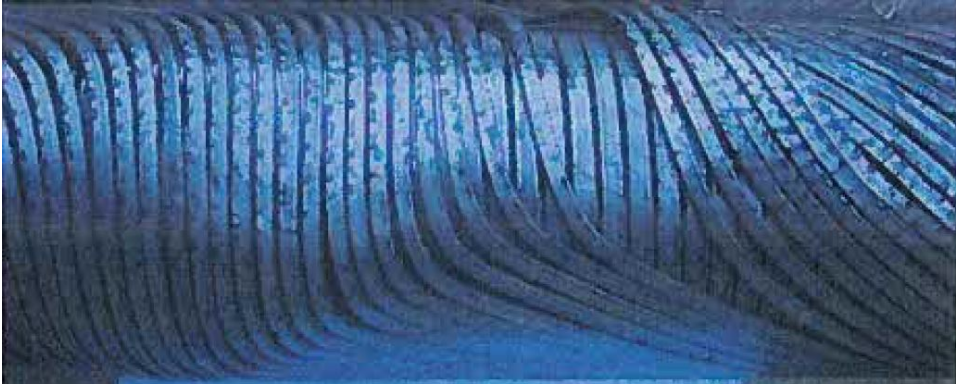
Figure 2.6: Example of lateral buckling of tensile armour wire [8].
