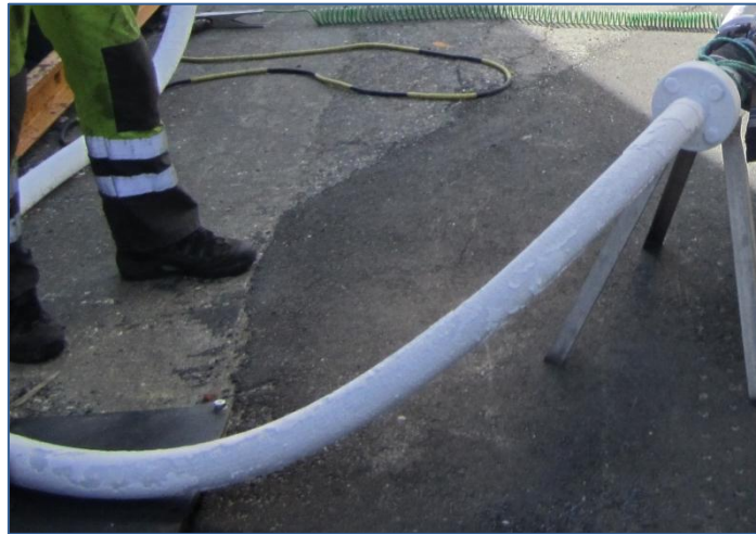
Figure 20 - Frozen bunker hose without insulation
