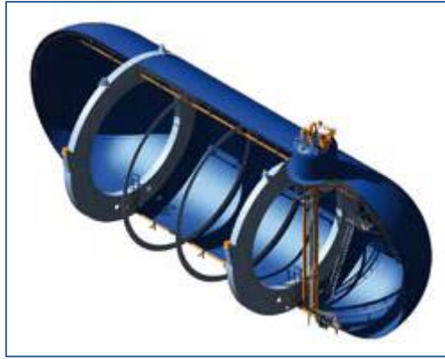
Figure 21 - Cylindrical IMO Type C LNG fuel tank
