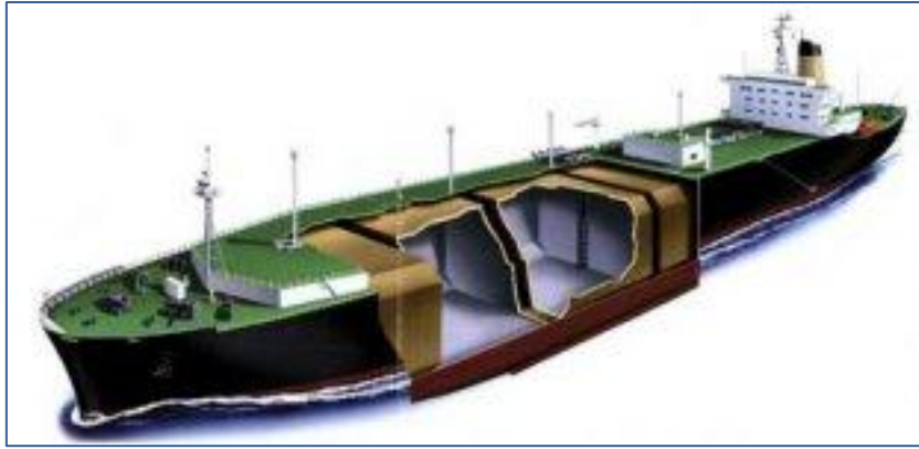
Figure 8 - LNG carrier with prismatic membrane containment system
