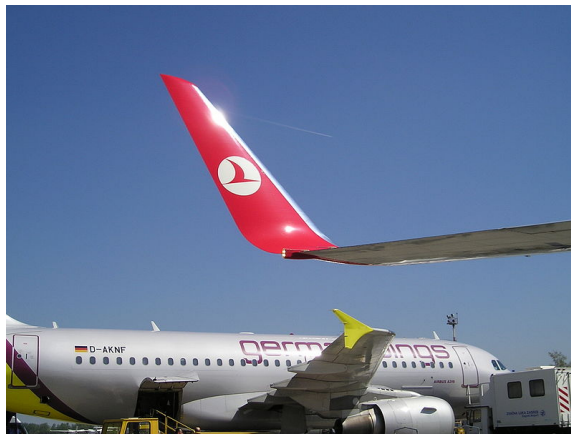
Figure 4.23: Example of a winglet on an airplane. From Wikipedia [30].
