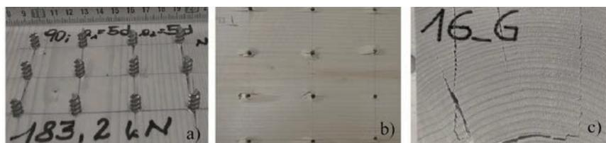
**Figure 3.3:** Failure modes of specimens (a) steel fracture, (b) withdrawal and (c) block shear [53]
