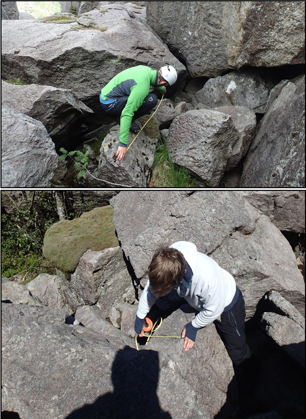
Figure 3.6: Examples of block size data-acquisition with measuring tape. Upper: measurement of a -axis. Lower; measurement of c -axis.
