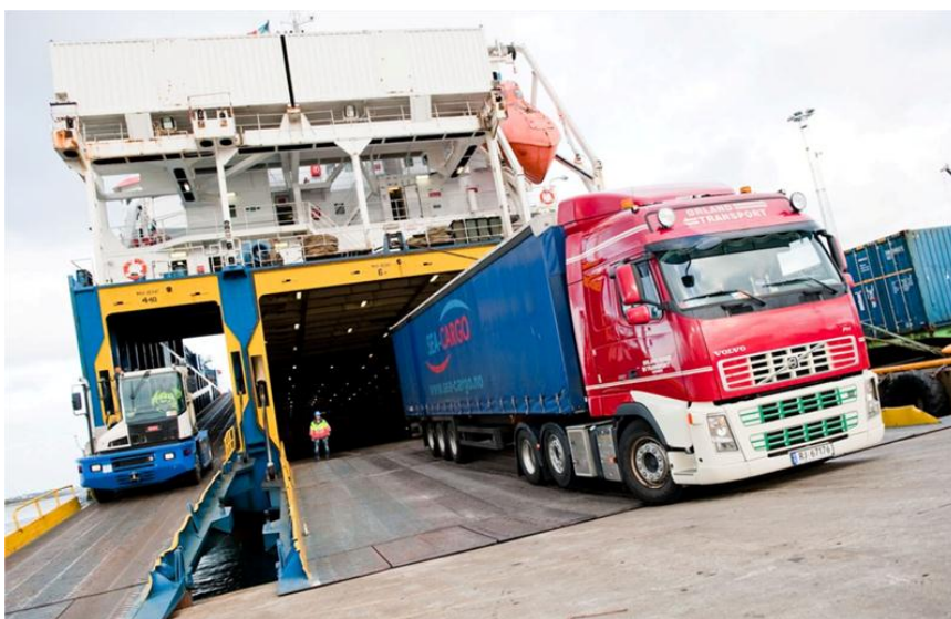
Figure 3.1: Truck with trailer being offloaded off a short-sea RoRo-ship [15].
