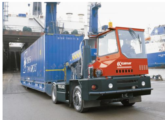
Figure 3.2: Terminal tractor discharging a container on a cassette [17].
