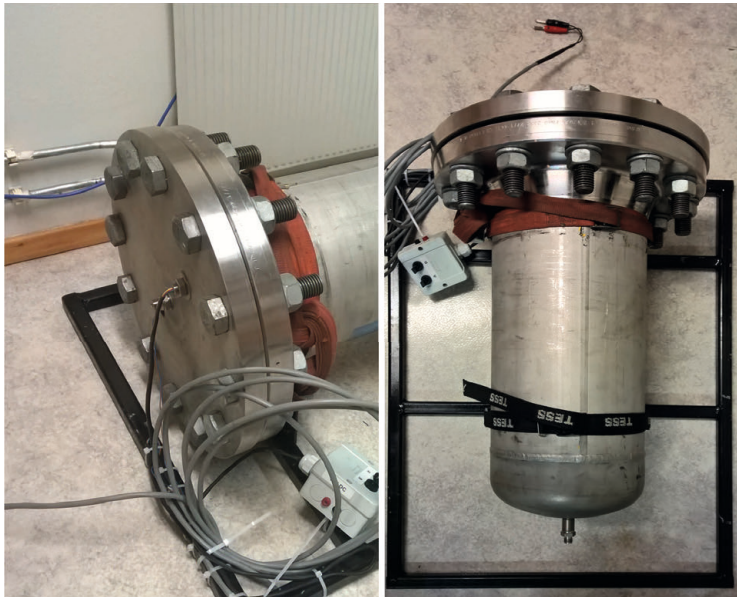
Figure 3.5: The pictures show the water hose connections at each end of the tank, and the dry side of the bulkhead-mounted sensors in the lid.
