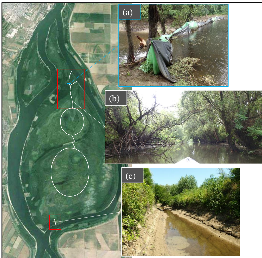
Figure 13. Areas of main interest for the hydraulic computations (Google Earth, 2014) (a) weir structure in the Hogioaia-channel, (b) Hogioaia-channel between lakes and weir, (c) LIFE-channel (Pictures: Zinke & Aberle, 2015). The lakes and their connection channels are simplified as circles.
