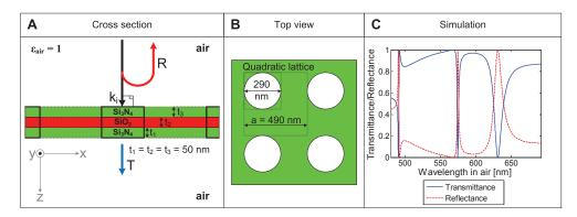
Fig. 2. (A) Cross section and (B) top view of the designed photonic crystal membrane. (C) Simulated transmittance and reflectance for a normal incidence plane wave is given as a function of wavelengths from 490 to 692 nm.
