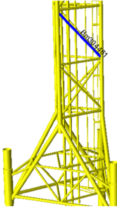
Figure 5.8: Location of element 304461 in the 3L-jacket
