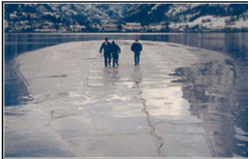
Figure 10.1 Nordic water Bag with volume of 10.000\text{ m}^3 for transport of Fresh water. Picture taken during full scale test in Sognefjorden
