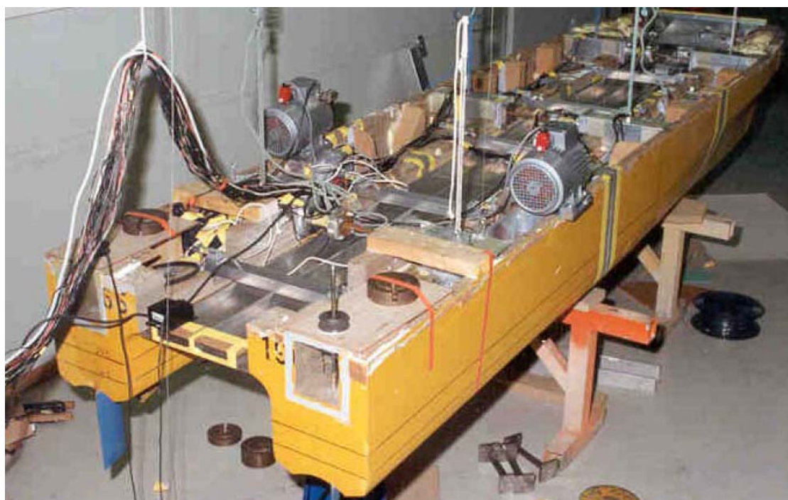
Figure 7.6 Hinged model of an elastic catamaran
