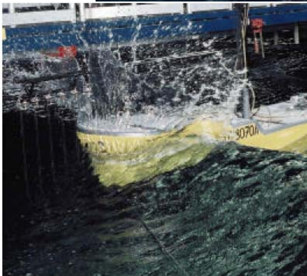
Fig 4.3 Photo showing wave impact damage to bow of Schiehallion FPSO on UK sector and model testing of bow slamming incident for the same case
