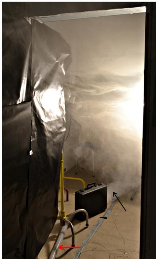
Figure 43. The warm zone filled with the smoke during the smoke test operation. Discharging point is marked with black arrow.
