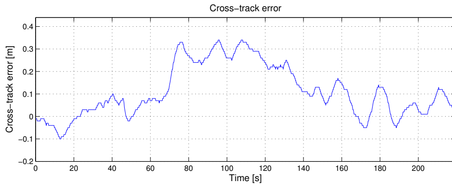
Figure 4.46: The cross-track error increases when the ROV follows a circular path.
