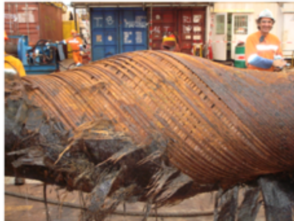
Figure 2.7: Birdcaging of riser, given by SRT
