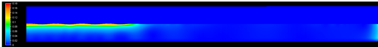
Figure 4.10: Contour plot of superficial water velocity at t=5s . Red indicate maximal velocity [ 0.2m/s ] and blue indicate zero velocity [ 0m/s ].
