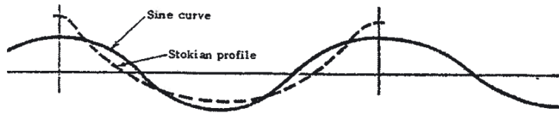
Figure 3.4: Comparison between Stokes and Linear wave profile (From Myrhaug (2006)).
