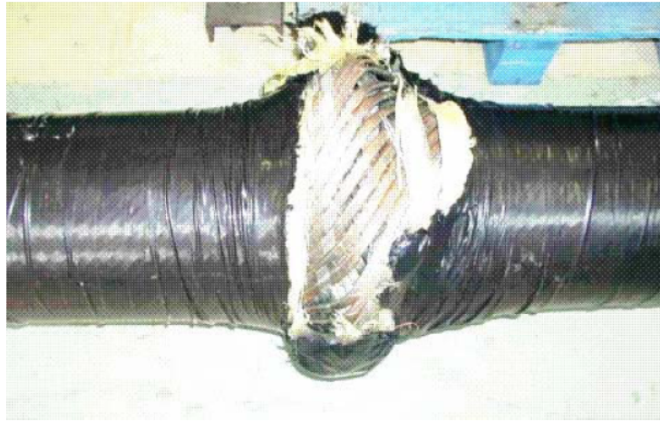
Figure 4: Bird-cage failure of flexible pipe [4].
