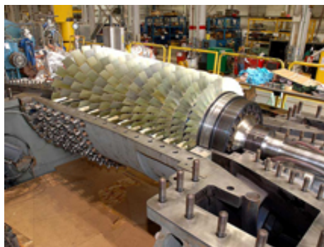
Figure 2.3: Picture of an open axial gas compressor.
