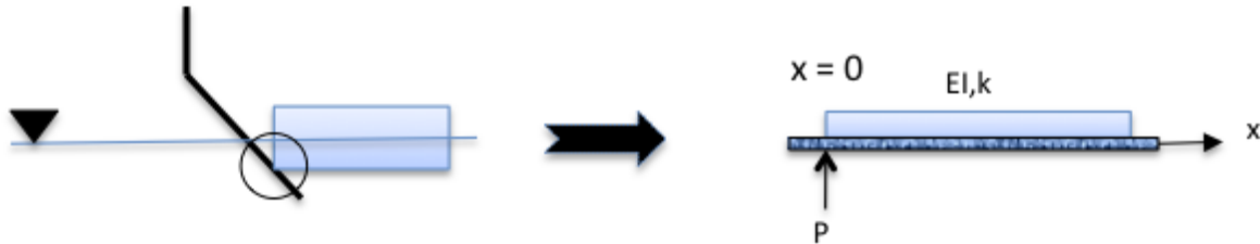
Figure 5.14: Simplified model for ice-structure interaction
