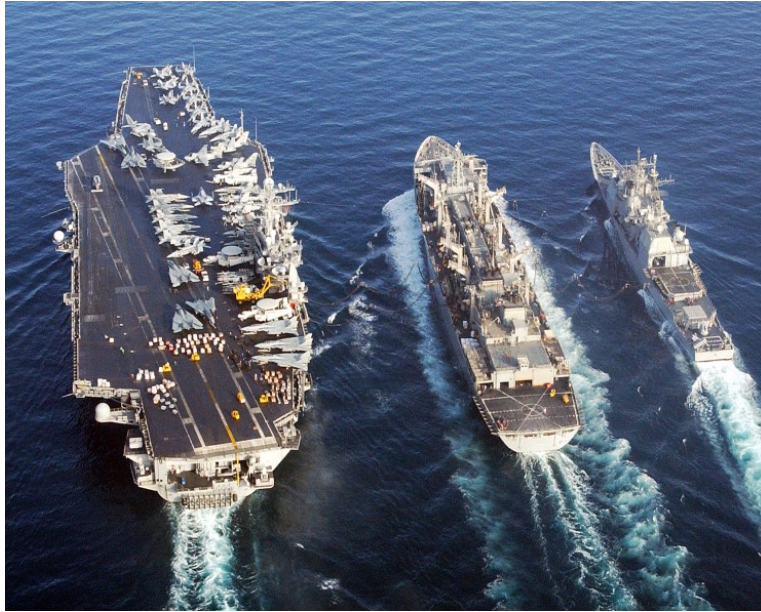
Figure 1.2: USS Harry S. Truman CVN-75, USNS Arctic T-AOE-8 and USS Monterey CG-61 performing an underway replenishment in the Persian Gulf. Courtesy of MaritimeQuest (2010).
