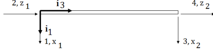
Figure 5.6: The riser element modeled as a bar element with four DOFs. x is transverse of the element, positive to the right, and z is along the element, positive upwards.
