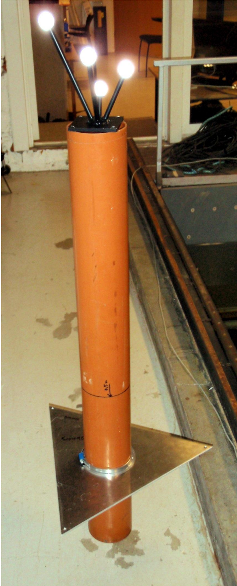
Column with mooring plate and motion reflectors
