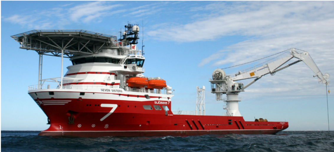
Figure 3.1: Seven Sisters with the AHC knuckle jib crane in operation. Courtesy of Subsea7 (2011).
