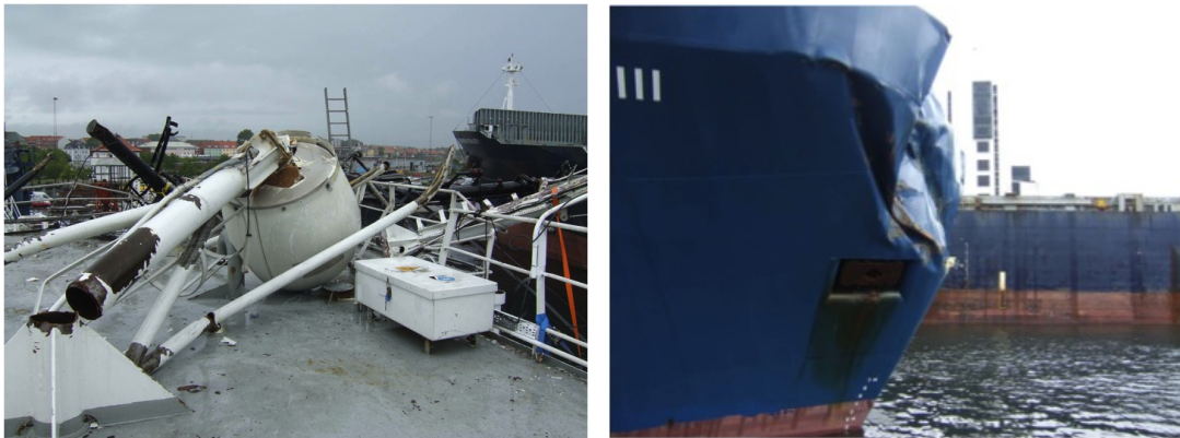
Figure 2.7: Left: Vessel equipment torn off. Right: Bow pushed in, from side
