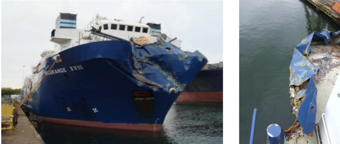
Figure 2.6: The damaged bow of Big Orange
