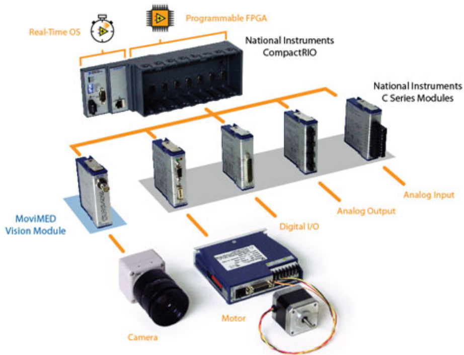
Figure 8.1: Hardware configuration example. Illustration: National Instruments
