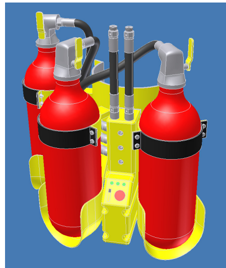
Figure 26: The multi directional electronically actuated valve, also called the control valve, mounted on the bottle rack along with hoses, bottles and connectors.
