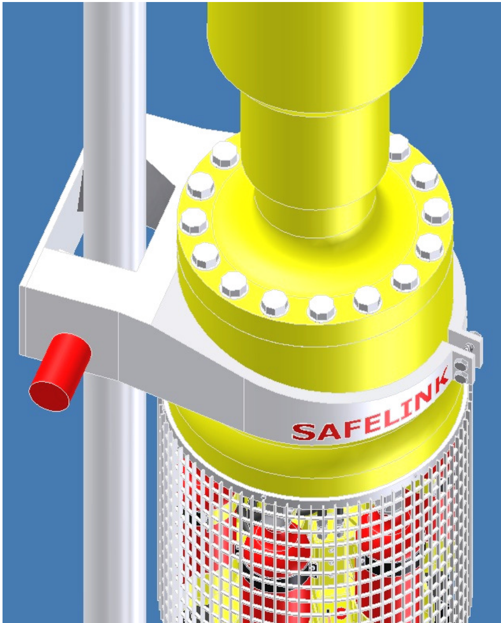
Figure 59: The cutting system mounted on the bottom connector. The umbilical line passes through the cutter.
