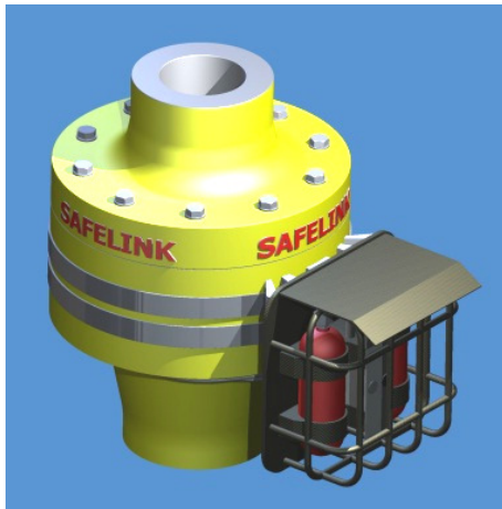
Figure 4: The preliminary project thesis final design. Pressure batteries are placed outside in a protective housing. The interface to other riser joints has not been decided upon.
