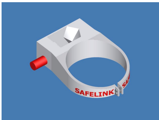
Figure 57: The mounting ring with the cutting system attached.
