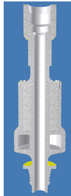
Figure 9: The section view of the SL design, presenting the integrated pressure batteries.
