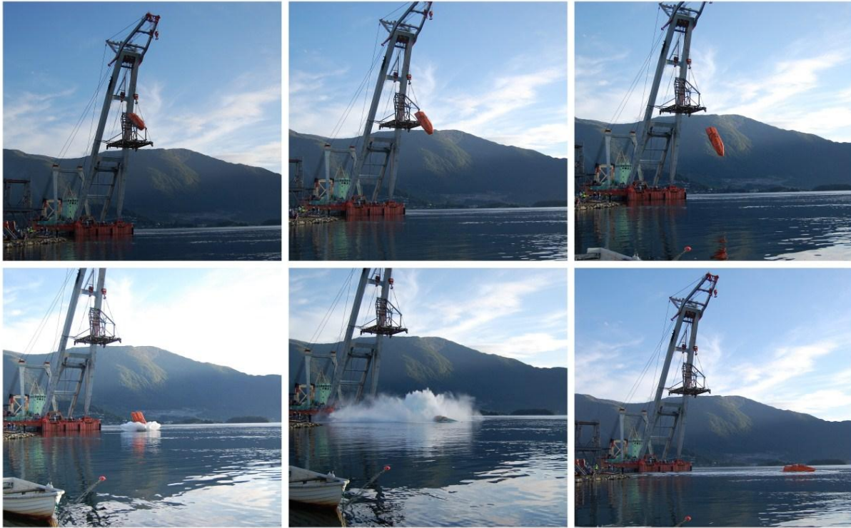
Figure 18: Full scale free fall lifeboat trial. Photo: Kristian Nedrevåg
