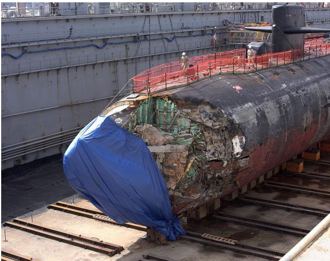
Figure 12 USS San Francisco after collision with an underwater mountain (33)
