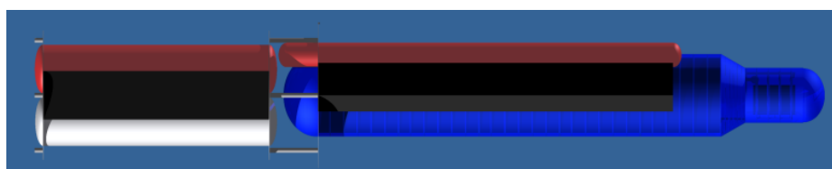
Figure 33 Side view of the main ballast tanks
