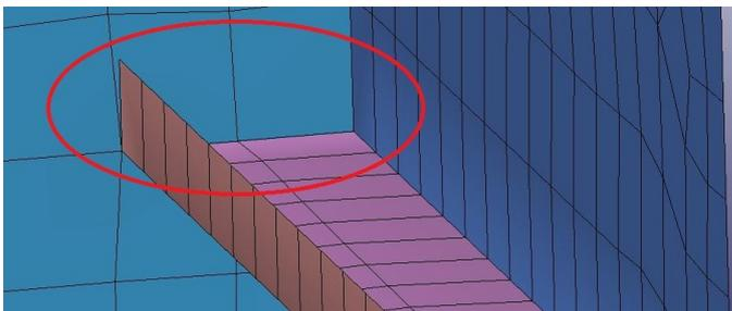
Figure 11: Stiffener passing through frame
