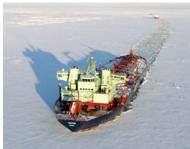
Fig. 1.3 A DAT crude carrier, MT Tempera, owned by Neste Oil and built by Sumitomo Heavy Industries in 2003 (Jones, 2004)
