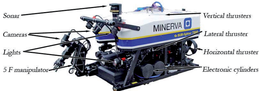
Figure 3.2 The Minerva ROV and its main components. An electric manipulator has been mounted after this picture was taken.
