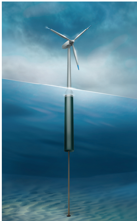
Figure 2.4: Tension leg spar wind turbine ( CeSOS Annual Report 2009 ).
