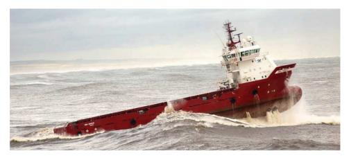
Figure 1.1: Supply vessel operating in heavy sea, where the emersion of the tunnel thrusters on the bow can be observed. Courtesy of Rolls-Royce Marine (RRM).
