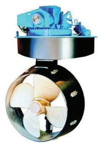
(a) Ulstein Aquamaster azimuth thruster.
