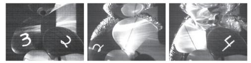
(a) First impact of the propeller on(b) First impact of  $Blade_1$  on the(c) Minimum blade thrust, t = -the free-surface, t = -0.1388 s. free-surface, t = -0.0972 s. 0.0805 s.
