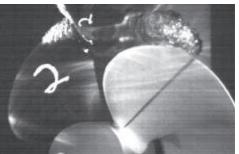
(b) Tip vortex: port and starboard, t = -0.1055 s.
