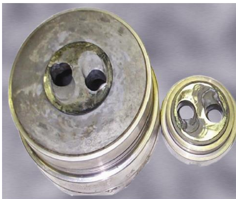
4-6: Example on sand erosion of a MOV choke
