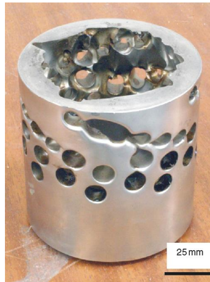
4-7: Example on an eroded cage
