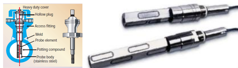
6-2: A sand erosion probe with 4 probe elements installed in a pipeline (left) and how they look (right)
