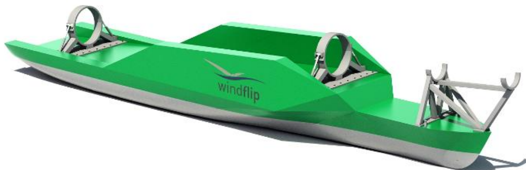
Figure 36 Sketch of fastening mechanism during transit
