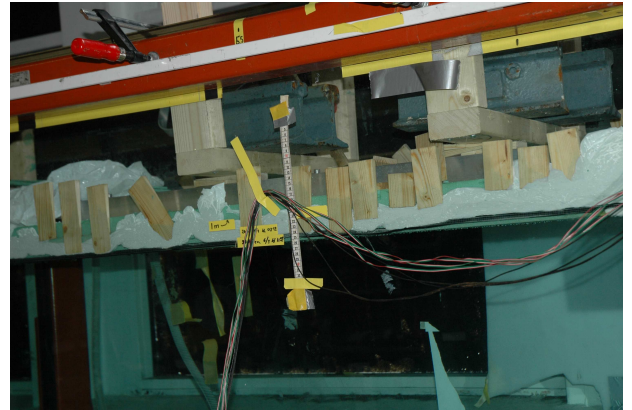
Figure 5.9: Rubber list and plastic bags forced between the ice and glass wall.
