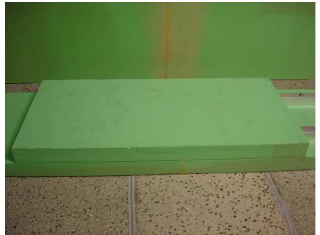
Figure 5.2: Upper: Ship-section model, on the left it is seen from the front and the right from the side, the copper tape makes a wave-gauge in two pairs i.e. two wave-gauges. Lower: the two divynycell plates that makes the artificial ice.
