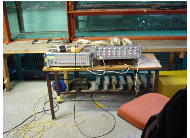
Figure 5.4: Upper: To the left the actuator with the force gauge mounted and a aluminum frame to hold a model. To the right the actuator control unit with emergency stop button on top. Lower: on the left wave-gauge for far-field wave elevation registration and in the lower right wave gauge amplifier (right) and signal amplifier for all measurement devices.
