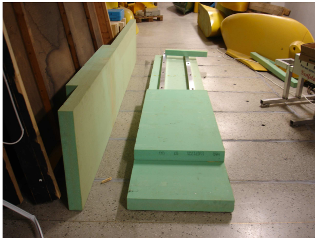
Figure 5.2: Upper: Ship-section model, on the left it is seen from the front and the right from the side, the copper tape makes a wave-gauge in two pairs i.e. two wave-gauges. Lower: the two divynycell plates that makes the artificial ice.
