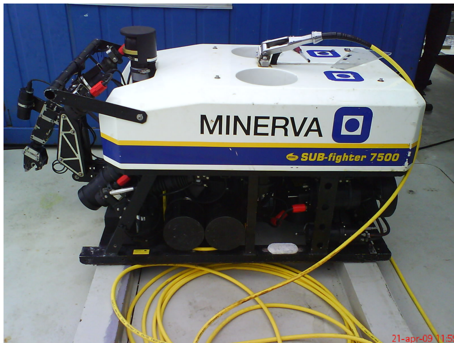
Figure 1: The NTNU ROV-Minerva.
