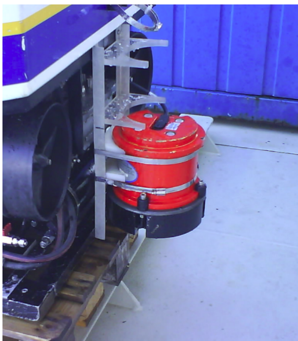
Figure 4: The DVL mounted on the rear of Minerva.
