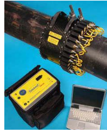
Figure 7 - Long range ultrasonic testing equipment (Scanning Technologies, 2007)
