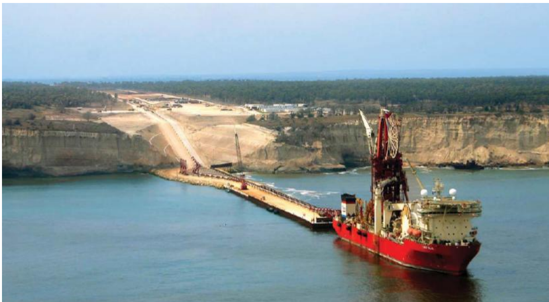
Figure 2.5 Technip’s DP Vertical Reel Vessel Deep Blue (J-lay) ( www.technip.com )
