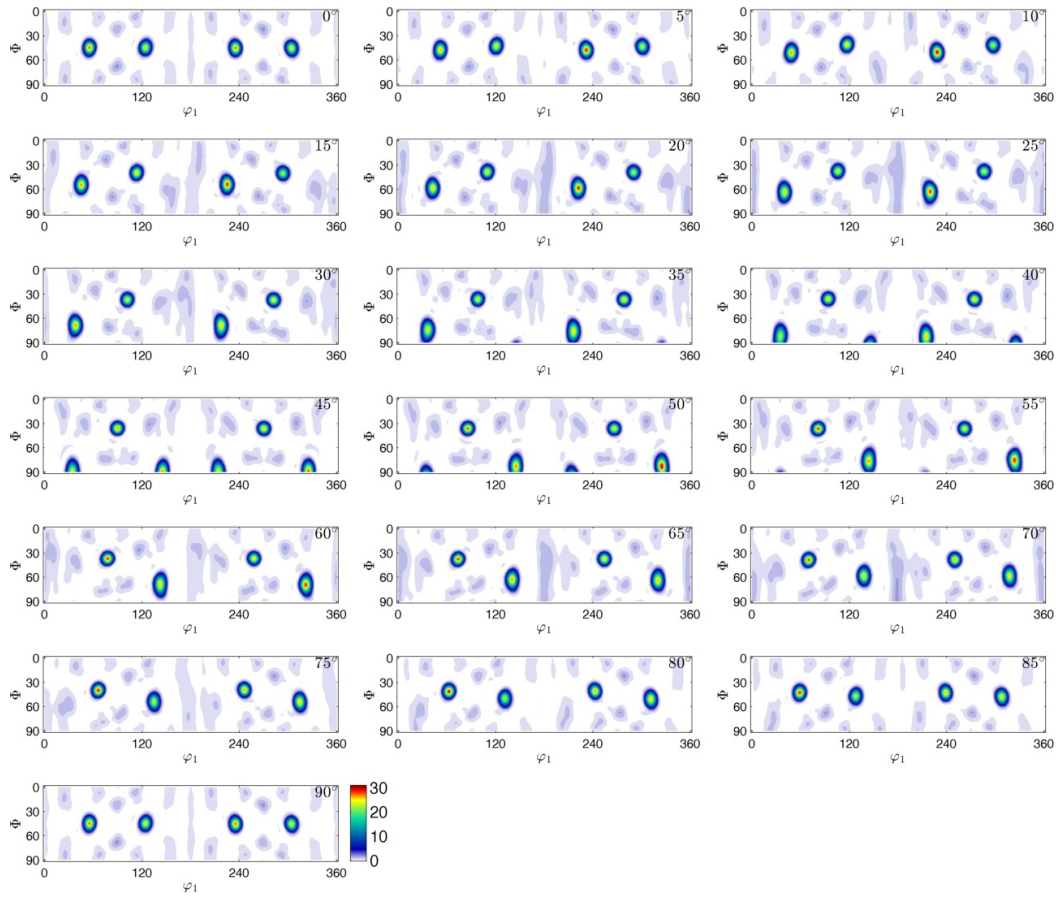
Figure D.11: Simulated ODF with 100% grain boundary nucleation
