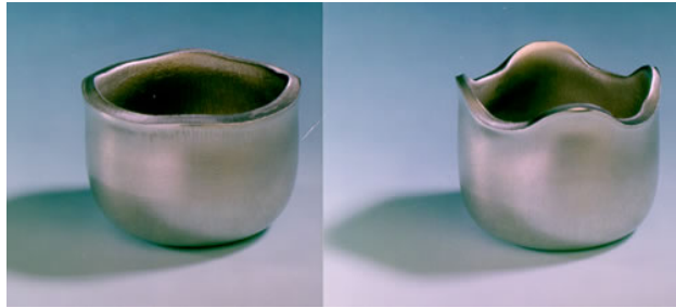
Figure 2.10: Effect of earing on deep drawn cups, strong texture to the right and weak to the left. The figure is taken from aluMATTER [17].
