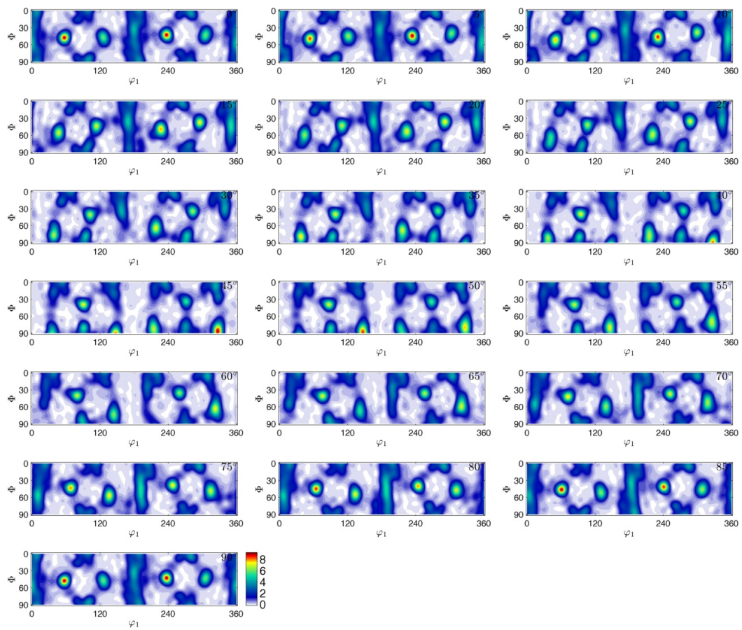
Figure D.4: ODF of heat treated D04 for 610s at 450°C
