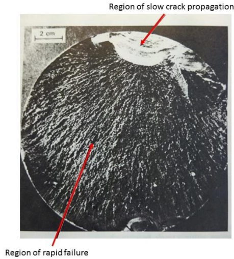
Figure 27: A fatigue fracture[31].
