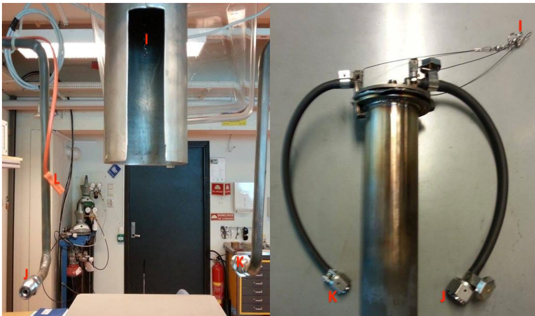
Figure B.7 TGA vertical retort furnace gas tubes (left) and crucible (right)
