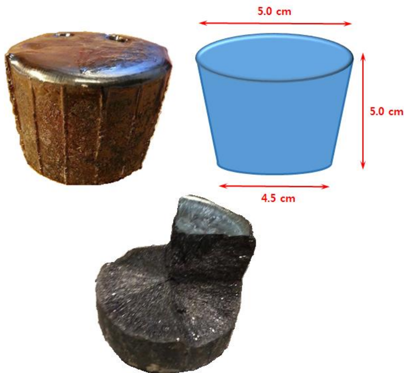
Figure 4.1 Bulk appearance (left) with sketch (right) & cross-section (bottom) of synthetic ilmenite
