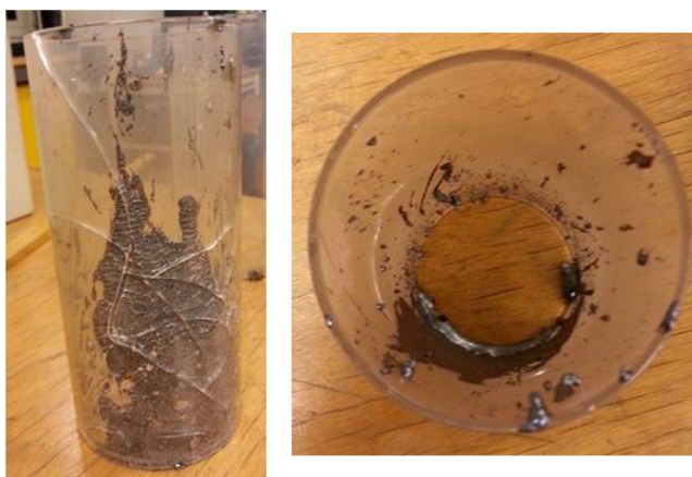
Figure B.1 Protection glass after splashing of the melt: rear view (left) and top view (right)
