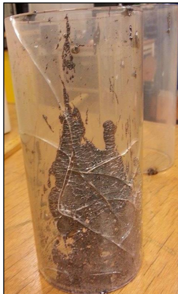
Figure 16: Splashing of liquid metal on protective glass.
