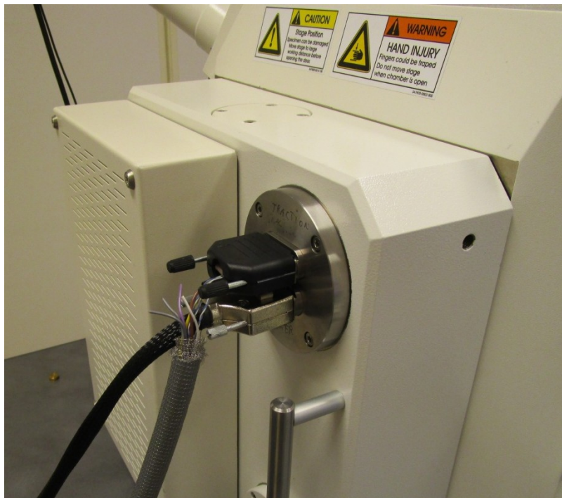
Figure B.19: Cables from hot stage controller and temperature logger connected to the SEM.
