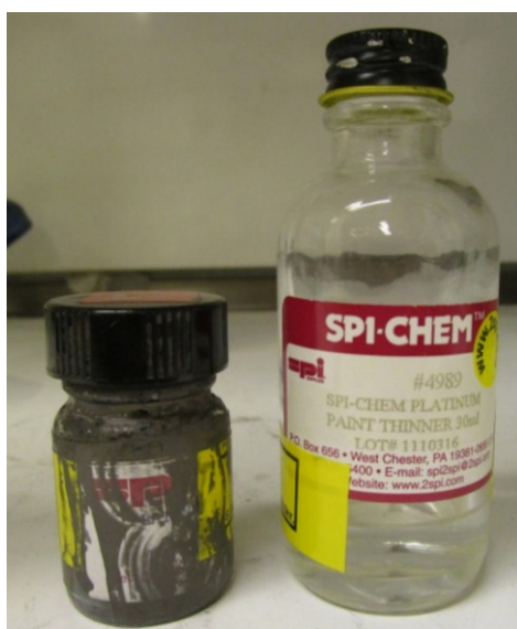
Figure B.9: The left bottle contains the SPI platinum paint and the right one a thinner that can be used to remove the paint already on the furnace.
