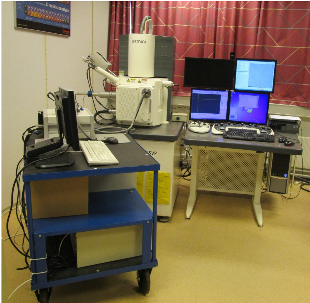
Figure 3.5: Zeiss Gemini Supra with in situ devices on the foremost table.
