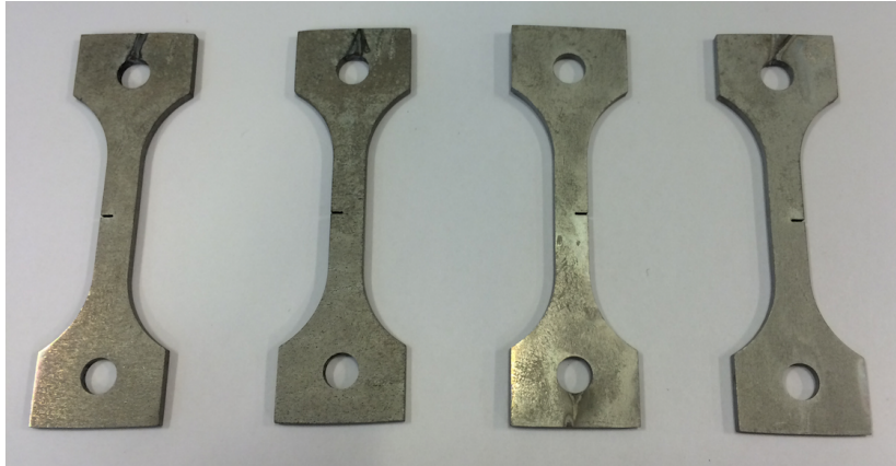
Figure 3.7: Image showing hydrogen pre-charged samples.
