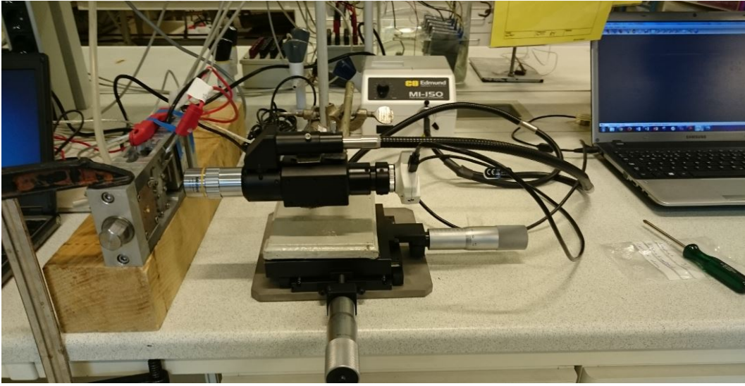
Figure 3.5: Experimental setup used for tensile testing with in situ cathodic polarization.
