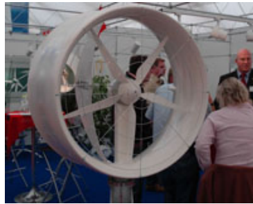
Figure 5.3: Diffuser-Augmented Wind Turbine (Wind-Works, 2010).
