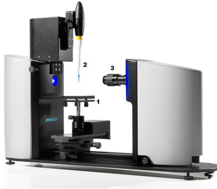
Figure 2.11: An optical tensiometer showing the (1) movable table on which the sample is placed, (2) the syringe from which a droplet is deposited, and (3) a recording camera. Adapted from the web pages of Biolin Scientific [41]
