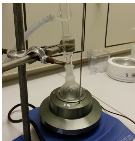
Figure 3.8: The experimental setup of the sol-gel synthesis. A 50mL round-bottom flask was put in a heating mantle, and placed on a hot plate with a magnetic stirring function. A water cooled cylinder was placed on the round-bottom flask in order to condensate evaporated solution.
