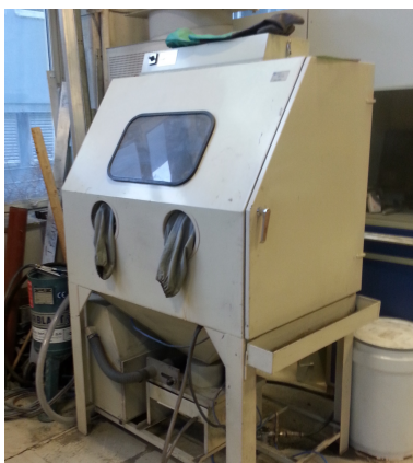
Figure 3.2: SINTEF's sand blasting cabinet in which micrometric roughness was induced.
