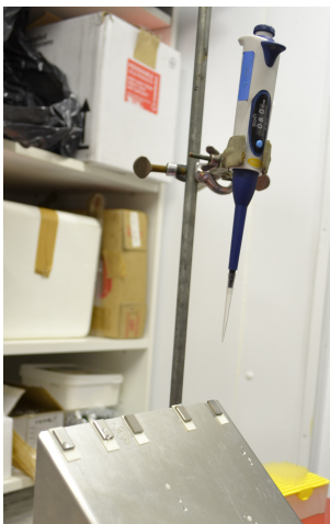
Figure 3.15: The experimental setup of the icing behaviour of a single droplet. The pipette was set to deposit 8 μL and held 5 cm above the samples. The samples were placed on a 45 °-tilted aluminium plate.
