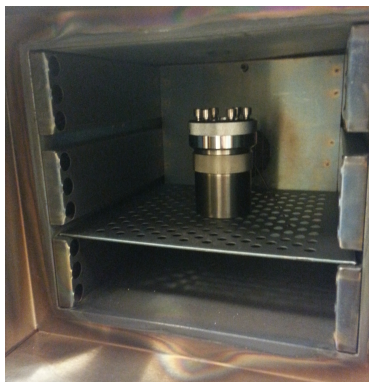
Figure 3.5: The placement of the autoclave inside the oven during growth of ZnO-NWs.
