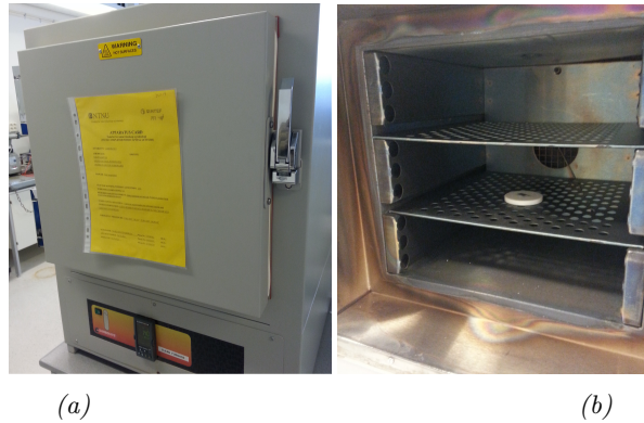
Figure 3.3: The oven, Carbolite 2 muffle furnace, and placements of the substrates inside the oven during heat-treatment. The samples were placed on an alumina-disc.
