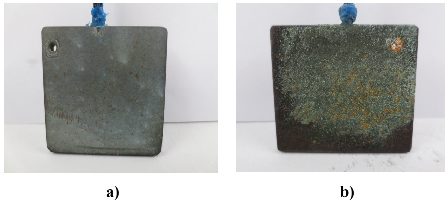
Figure 4.15 Sample appearance of freely exposed NAB after a) nine weeks of immersion in natural seawater, and b) followed by one week in 10 ppmW sulphide-polluted SSW without a MF.
