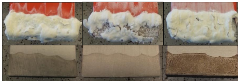
Figure 4-16: Pictures of 316-samples tested in artificial seawater at 1000 A/m 2 AC. The top pictures are prior to cleaning and the bottom ones are post cleaning. The left row was tested at -800 mV DC, the middle at -1050 mV DC and the right is the re-test of the middle one.
