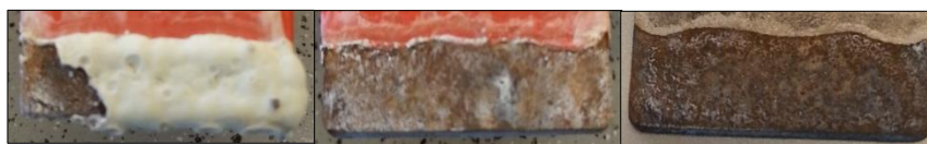
Figure 4-21: Picture of a 25Cr-sample before GIXRD analysis. It was tested in artificial seawater at -800 mV DC and 1000 A/m 2 AC. The left picture is just after the sample was removed from solution, the middle picture is before cutting and the right picture is after it was cut with water as cooling medium. This sample corresponds to the left pictures in Figure 4-18.
