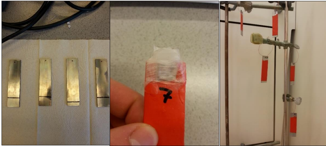
Figure 3-3: The left picture shows some samples before they were coated, and the difference in exposed area is visible. The picture in the middle shows how the sample top was covered to avoid unwanted corrosion. The right picture shows drying and storing of the samples after coating.
