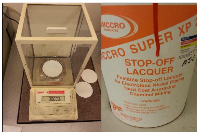
Figure 3-2: The left picture is of the standard analytical weight and the right picture is of the lacquer used to coat the samples.
