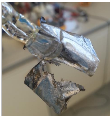
Figure 4-33: A photograph of the AC counter electrode that has started to dissolve.
