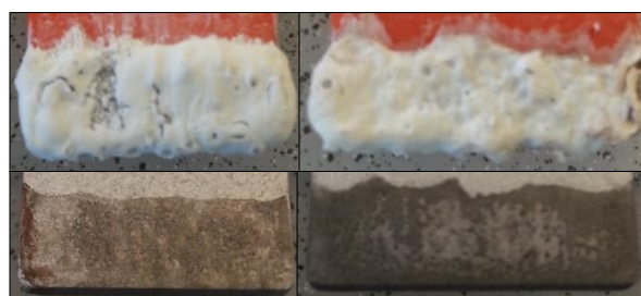
Figure 4-18: Pictures of 25Cr-samples tested in artificial seawater at 1000 A/m 2 AC. The top pictures are prior to cleaning and the bottom one is post cleaning. The pictures to the left are samples tested at -800 mV DC and the right at -1050 mV DC.
