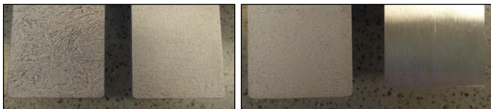
Figure 3-1: The first photo shows two 25Cr-samples, were the left one is prior to cleaning and the right one has been cleaned. The second photo shows the surface difference between some cleaned samples. The samples that was shiny, as the one to the far right was used for XRD and not weight loss measurements
