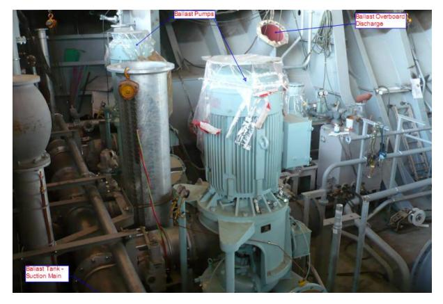
Figure 46: Ballast pumps and piping
