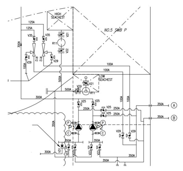
Figure 32: P&ID of cement carrier ballast system
