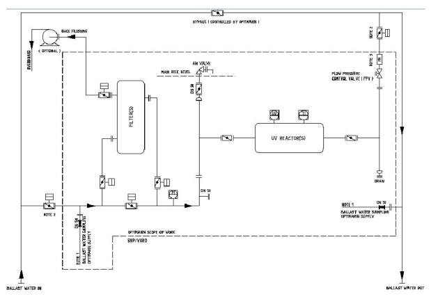
Figure 20: OptiMarin Ballast System flow diagram [12]
