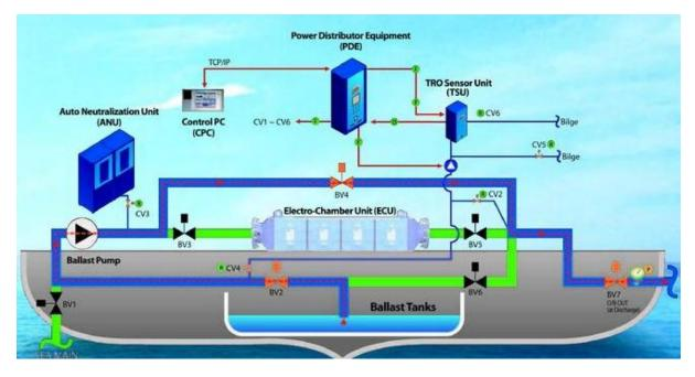
Figure 31: Electro-Cleen flow diagram during discharging [15]
