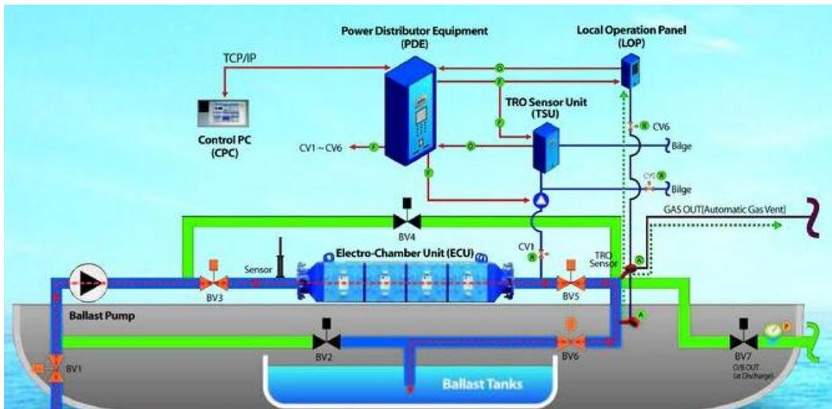
Figure 29: Electro-Clean flow diagram [15]
