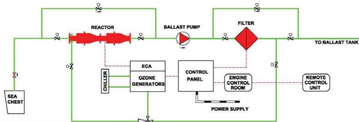
Figure 33: WSE Unit flow diagram [16]
