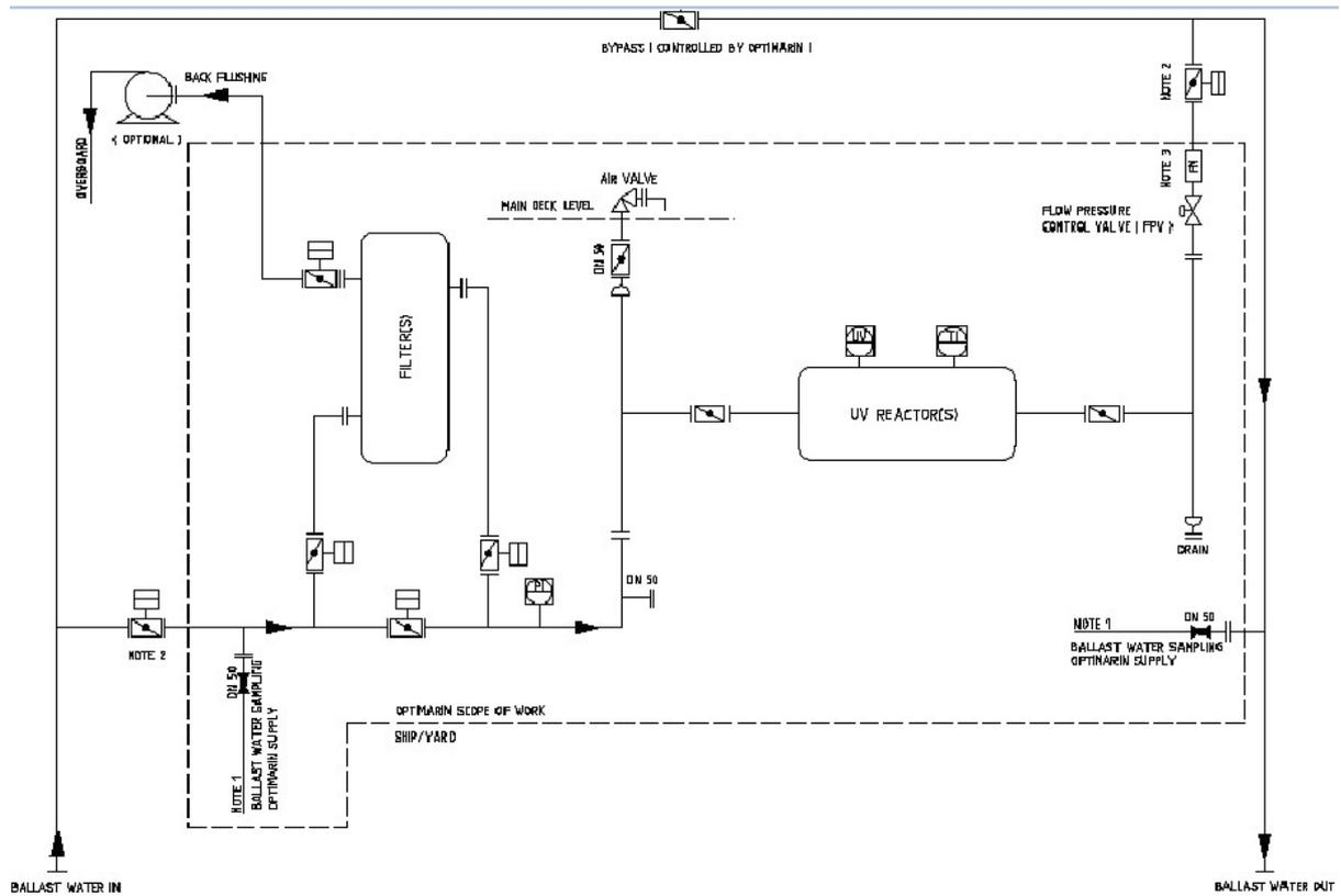
Figure 20: OptiMarin Ballast System flow diagram [12]
