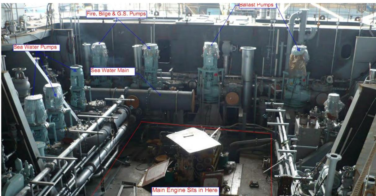
Figure 43: Tuju Arrow ballast pumps
