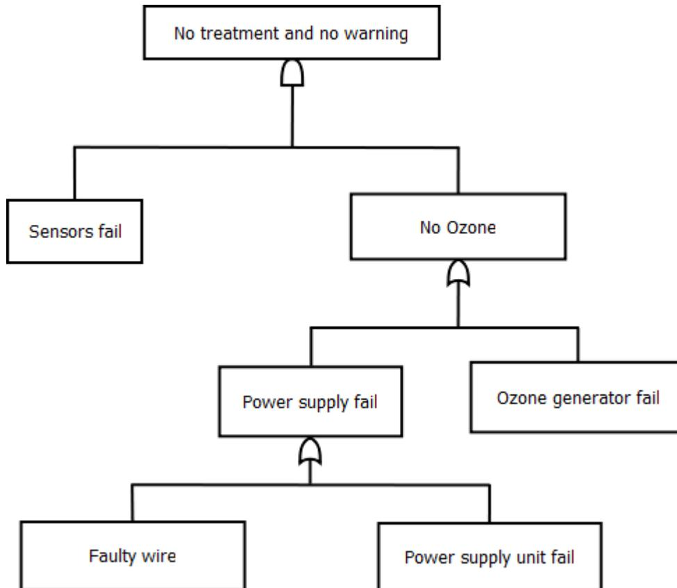
Figure 38: BlueBallast fault tree
