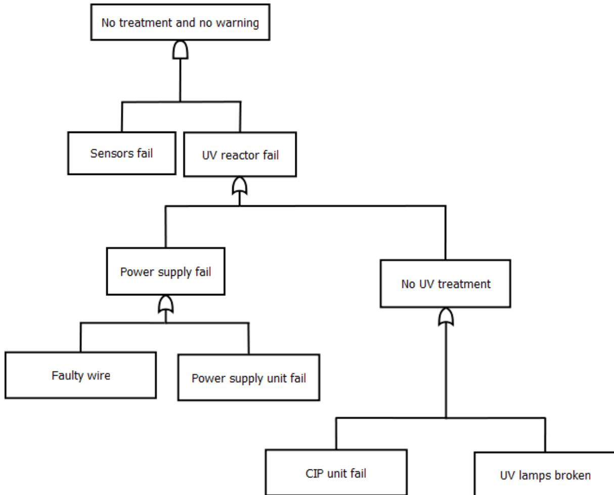
Figure 25: Alfa Laval PureBallast fault tree
