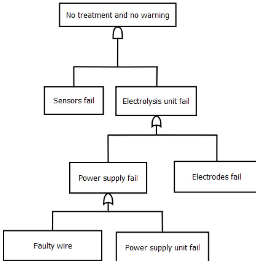
Figure 30: Electro-Cleen fault tree
