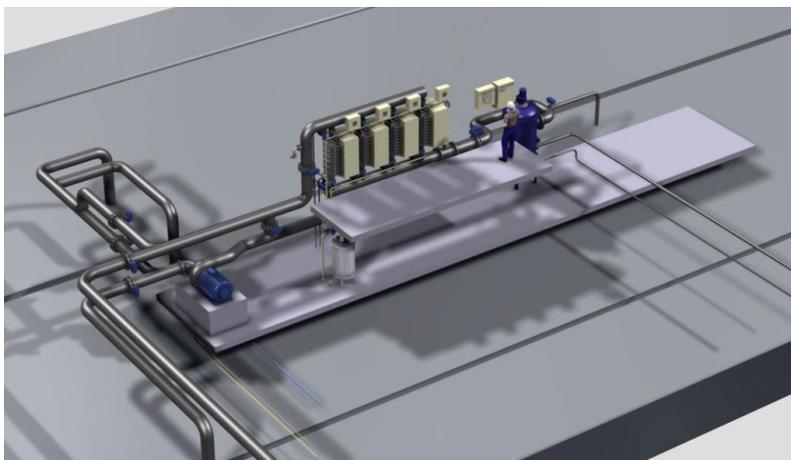
Figure 23: 3D model of PureBallast with piping
