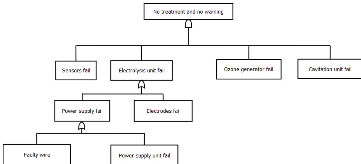
Figure 36: WSE Unitor fault tree
