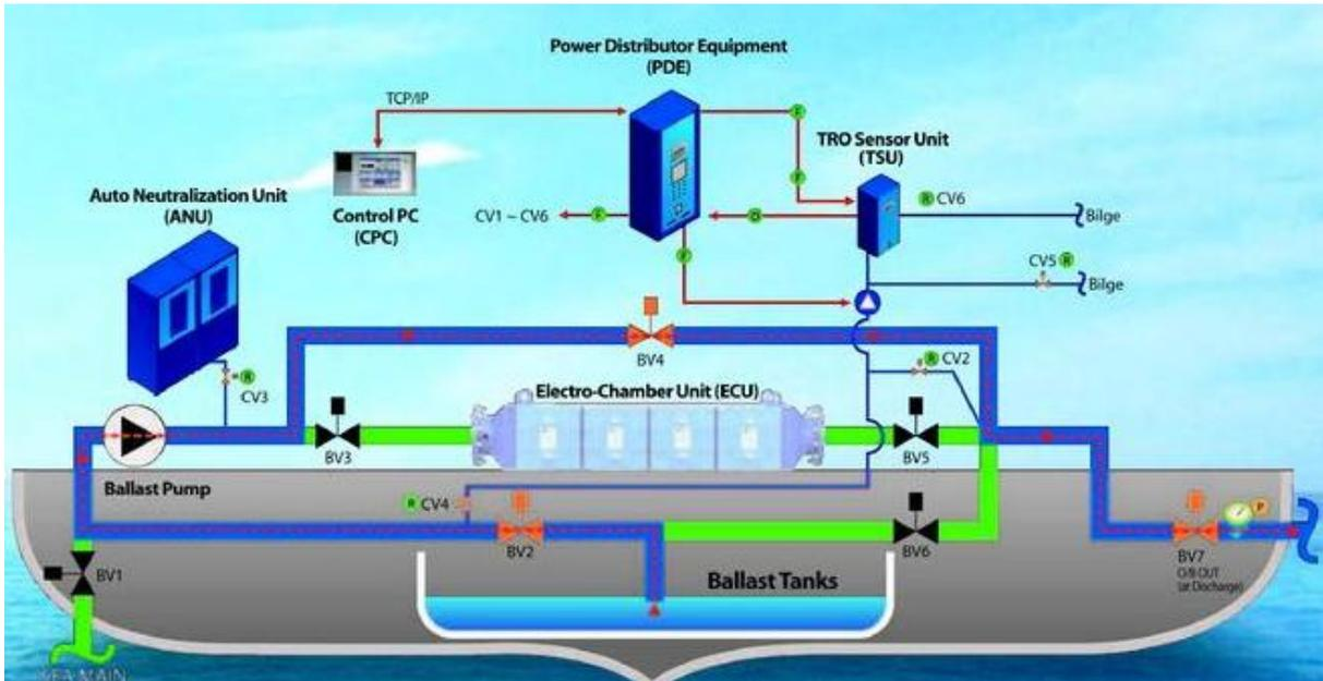
Figure 31: Electro-Cleen flow diagram during discharging [15]
