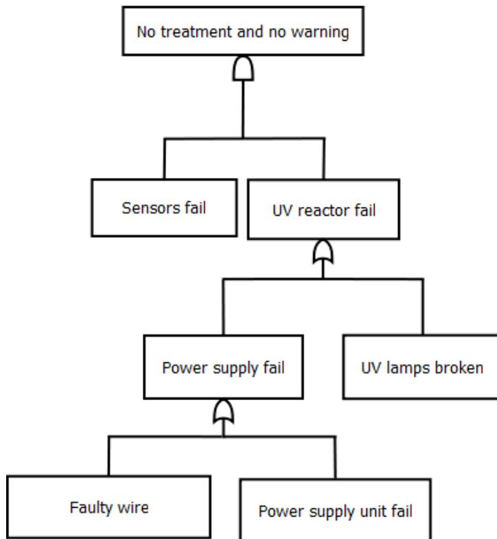
Figure 21: OptiMarin Ballast System Fault Tree
